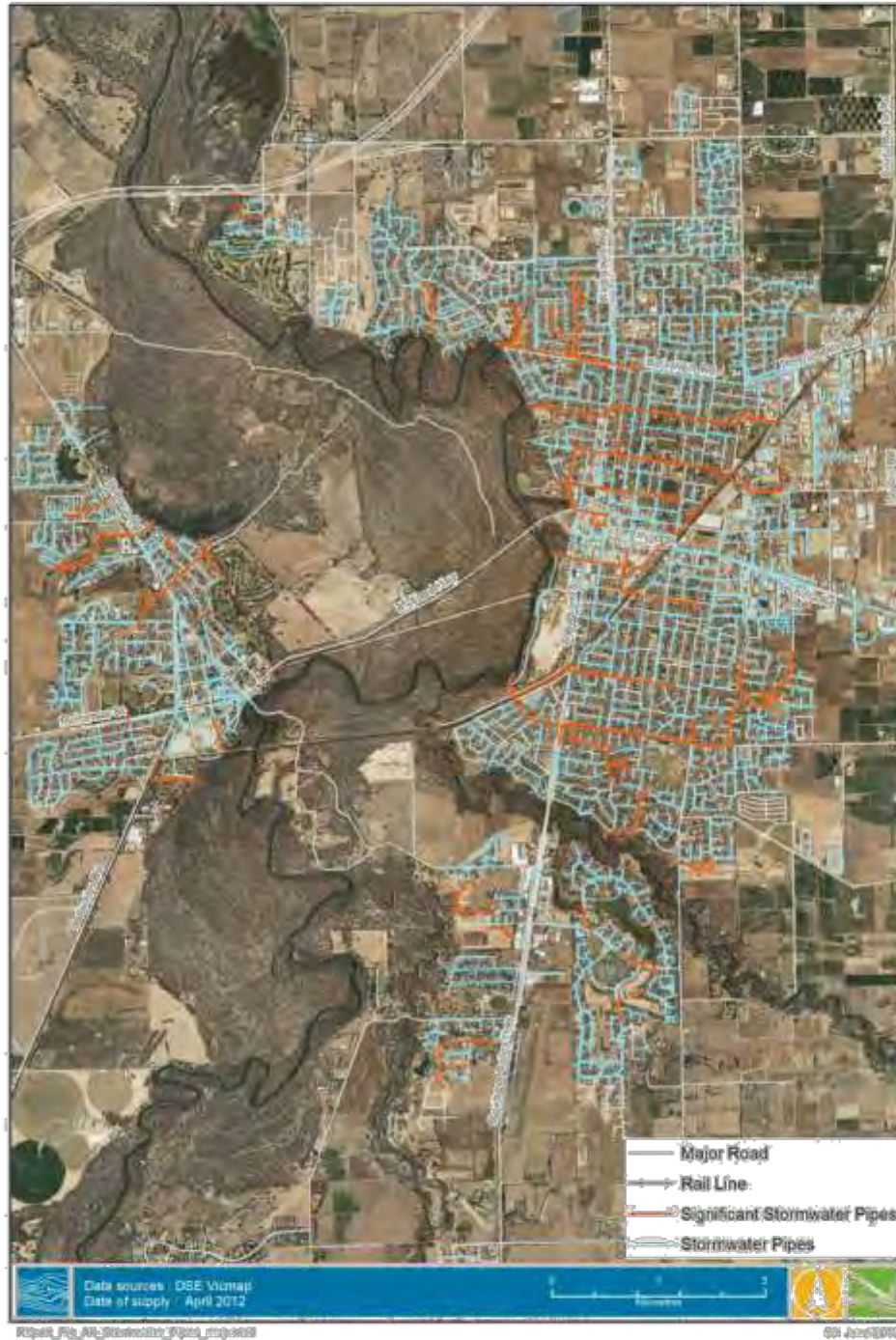
FIGURE 3-6 SHEPPARTON-MOORoopna STORMWATER PIPE SYSTEM
