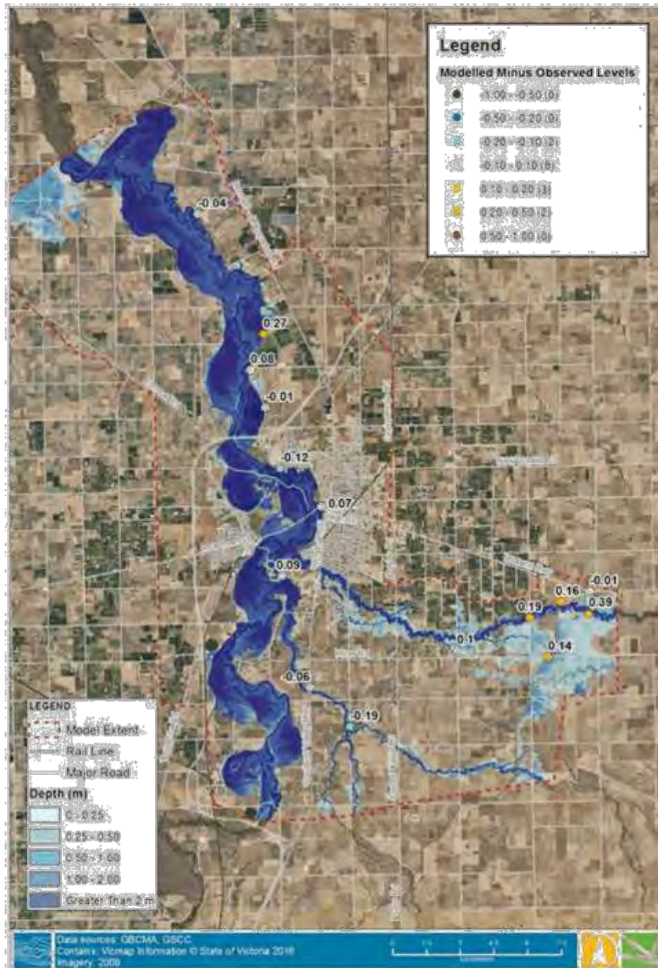
FIGURE 5-9 HYDRAULIC MODEL CALIBRATION PLOT – SEPTEMBER 2010
